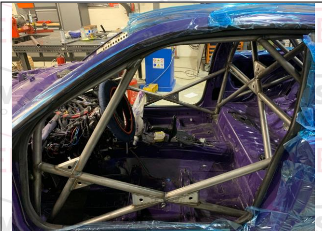
PHOTO 10 ANTI-INTRUSION DOORBAR - DRIVER
