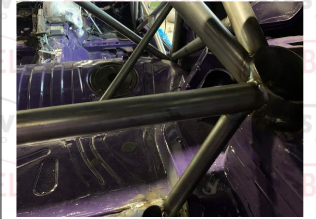
PHOTO 12 SHOULDER HARNESS ATTACHMENT - DRIVER
